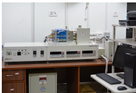
Seebeck Coefficient Measurement
