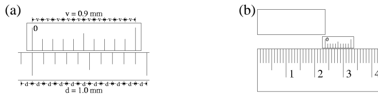
Figure 1(a) Direct Vernier (b) measuring the length of the rectangle using a direct vernier scale
