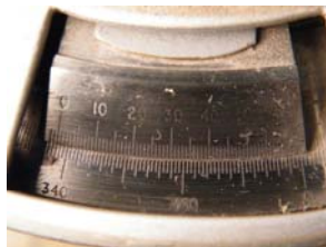
Fig. 7 Typical vernier to circular scale of a spectrometer
