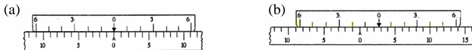
Figure 4. (a) Extended Vernier (b) measuring the length using an extended vernier scale (note the arrow)
